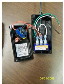
Remove the front cover to expose the wiring and the mounting screws.
