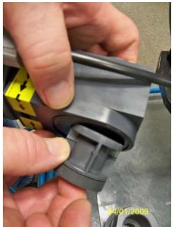
Insert the check valve assembly into the valve body.
