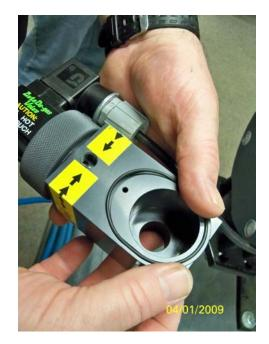
Install the lower O-ring to the valve. (Note- a small amount of light grease applied to the O-rings will help keep them in place during installation.)
