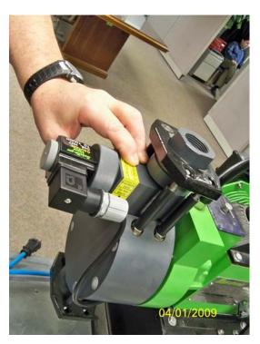
Replace the valve cap and tie bar.
