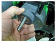
17. Slide the solenoid over the Core Tube and secure with Cap Nut. Hand Tight.
