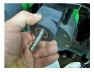
5. Remove Core Tube Assembly.
