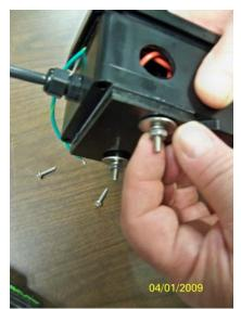
Remove the two nuts, lock washers and flat washers.
