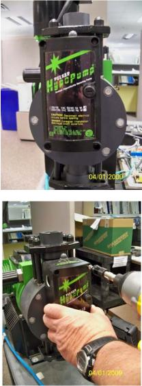
Remove the front cover from the old Hypo valve enclosure.
