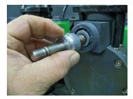
6. Remove outer spring from Core Assembly (Seal Kit Assembly) and pull Core Assembly out.
