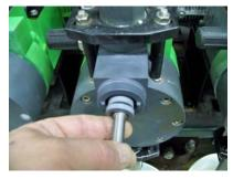
14. Install new spring over Core and check that Small Spring is still in the Core.
