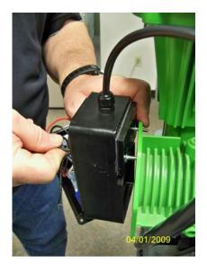
The existing top two holes in the rib of the gear box will line up with the holes in the electrical enclosure. Use a 3.0 mm Allen wrench to tighten the mounting screws, and a 9 mm open end wrench for the nuts.
