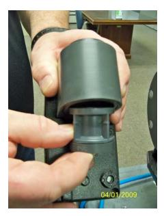
Remove the check valve assembly.
