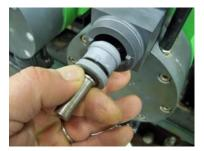
7. Inspect Valve Body for O-rings that may have been left in and remove.
