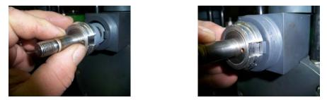
16. Slide Union Nut over Core Tube and tighten onto Body. Do not over tighten, hand tight is sufficient.
