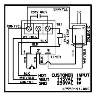
Wire the Hypo Valve AC power per the wiring diagram. Replace the front cover.
