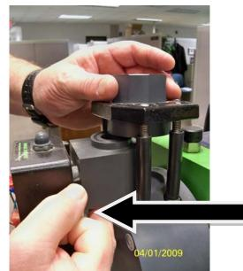
As you remove the assembly, remember to support the check valve so it does not fall out.
