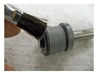
12. Apply a lubricant that is compatible with product being pumped to the Body O-ring and install into Valve Body.
