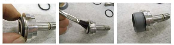
11. Install NEW O-ring on Seal Kit and with lubricant that is compatible with product being pumped.
