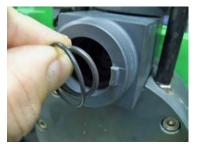
8. Remove the sleeve from the Core Tube and remove the O-ring.
