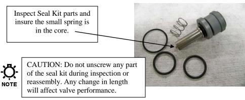
10. Install NEW O-ring onto core tube, lubricate with lubricant that is compatible with product being pumped, and reinstall sleeve over Core Tube.
