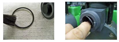
13. Install NEW Seal Kit into Valve Body. Use care to ONLY push straight into bore.
