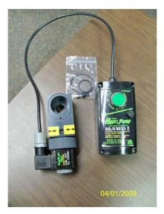
The new Hypo valve comes in three pieces, the valve body assembly with the solenoid, the electrical enclosure and the O-ring package. The solenoid and the electrical enclosure are prewired.
