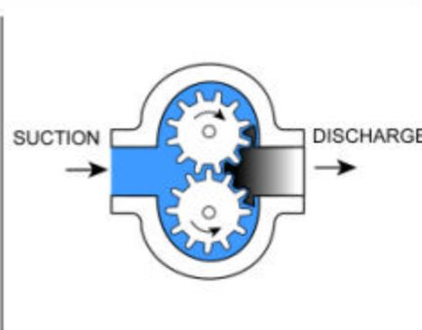
Fig 2. Rotary gear pumps are positive-displacement pumps operating to trap equal increments of fluid in the space between gear teeth and the pump housing for transport between intake and discharge ports.
