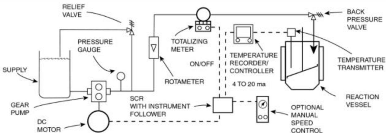
By design, it displaces a relatively constant volume per revolution and delivers essentially pulse-free linear flow. The quantity of fluid (flow rate) delivered to the process may be varied in three basic ways, with varying degrees of control sophistication:
