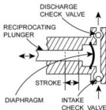
Fig 1. A pair of unidirectional check valves is required in the operation of reciprocating plunger and diaphragm pumps. Ball-check or disk-plate valves may be lightly spring-loaded to increase seating rate, but suction lift is reduced.
