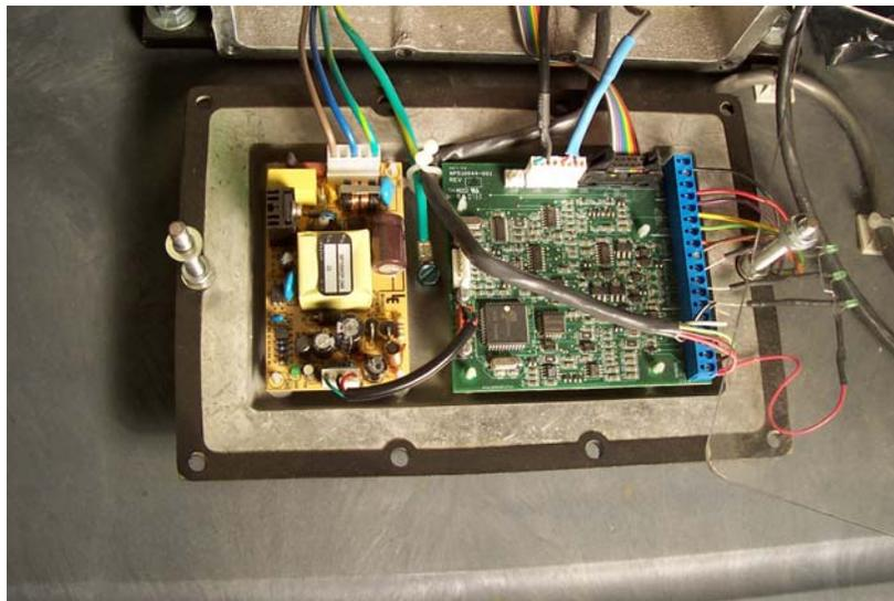
3. Remove black jumper wire from J17 to power supply by pulling straight up on connector
