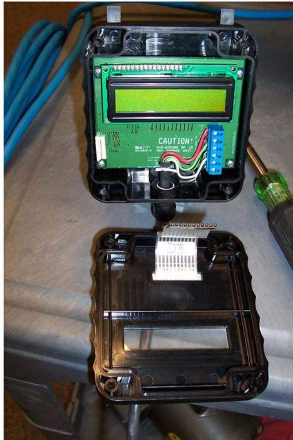
19. Remove the six wires from the blue terminal block mounted on the remote board.
